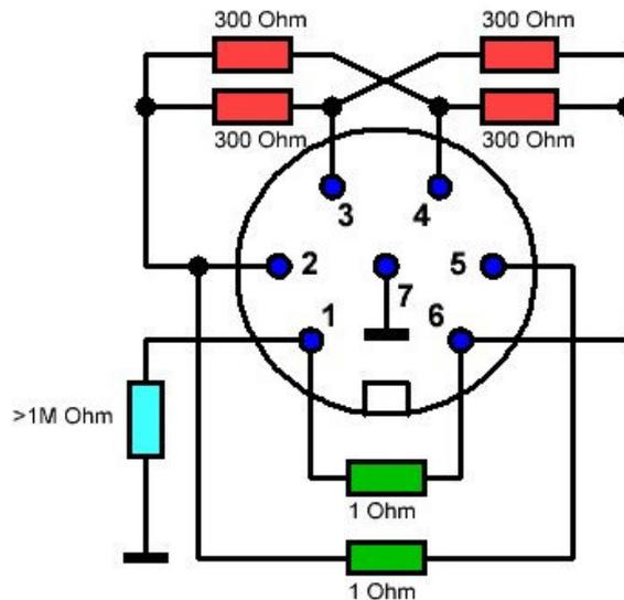
The absolute value of the resistors is less decisive and can be between 1 and 3 ohms for the 1 ohm values and between 200 and 500 ohms for the 300 ohms values, depending on the weighing cell type.
