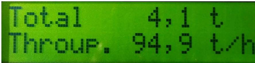
The last total weight generated and the current throughput are displayed. The total weight can be reset to zero at any time by pressing the blue **[Null]** key.
