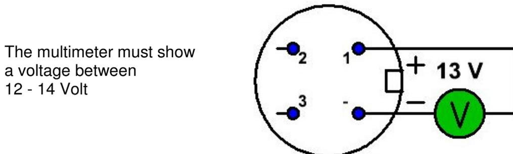
If this is not the case, check the pre fuse and the wire.
